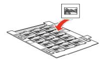
**Note:** The images and any wording on the slides should appear backward; the top of the images should face the open end of the slide holder. Do not cover any of the small holes in the slide holder.
